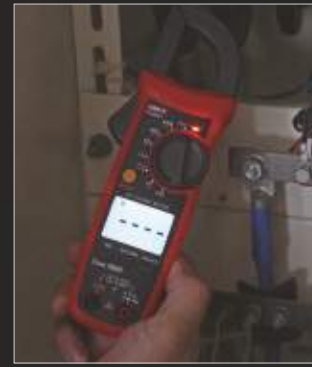
NCV multi-segment display and audio/visual alarm
