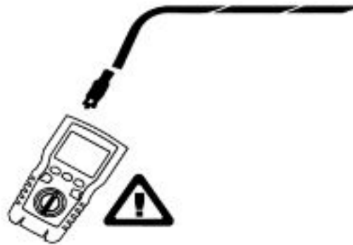
Figure 6.17 Voltage on Coaxial Cabling
