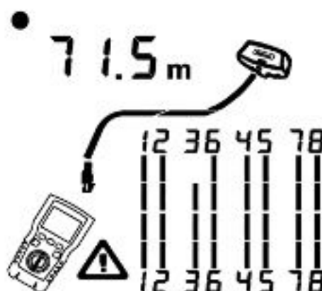
Figure 6.2 Open on Twisted Pair Cabling
