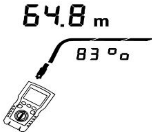
Figure 9.2 Determining a Cable's Actual NVP
