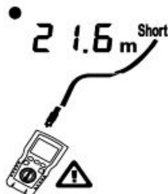
Figure 6.16 Short on Coaxial Cabling
