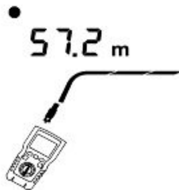
Figure 6.15 Open on Coaxial Cabling
