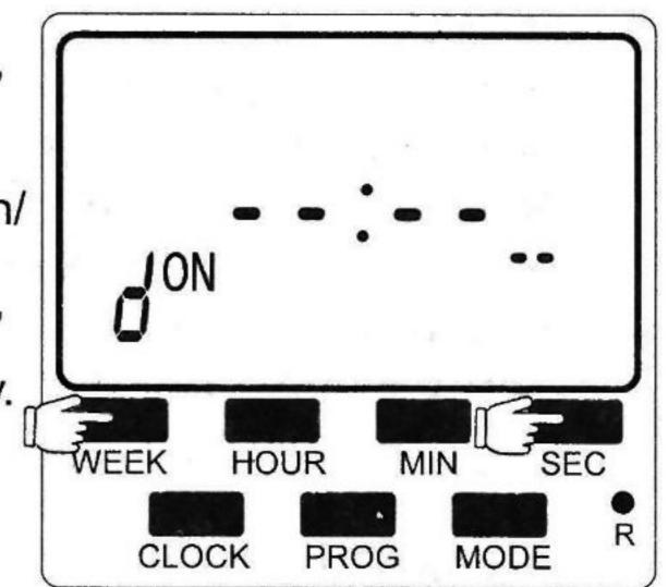
You can press "HOUR", "MIN" and "SEC" to set the Countdown/Loop time you want, the duration of Countdown/Loop can be set from 1S 99h59m. Press "MODE" to choose "ON" or "OFF" model of Countdown/Loop. Press "WEEK" and "SEC" again to exit the Countdown/Loop mode.
