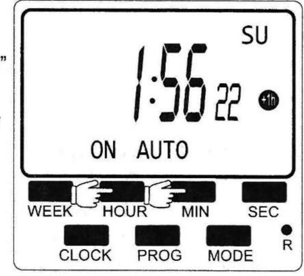
This function will allow the timer to adjust the current clock time on the timer by an hour ahead to accommodate daylight savings.
