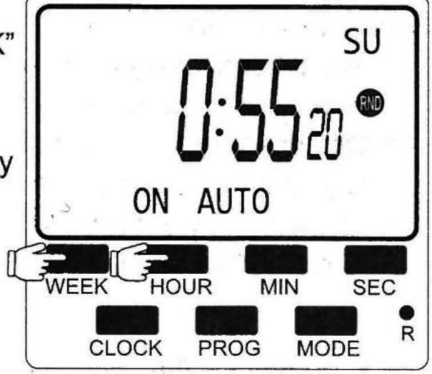
When start the random mode, the timer will turn on and off randomly with a 2-32 minutes variation based on the on and off schedule you set. The RANDOM function can only work in when timer is setting finish, and the time in auto mode. Press "WEEK" and "HOUR" again to exit the Random mode.
